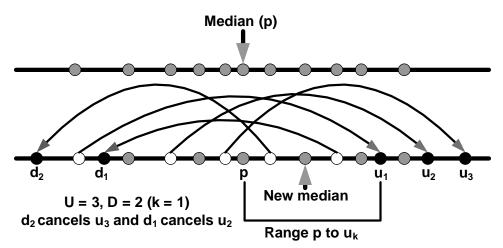
Fig. 2. Example showing how the values crossing the median can be canceled. The top line shows the distribution of sensor readings (grey circles) with the current median (p). The bottom line shows the new sensor values. If the new value differs from the old value, the old value is shown as a white circle and the new value is shown as a black circle.
