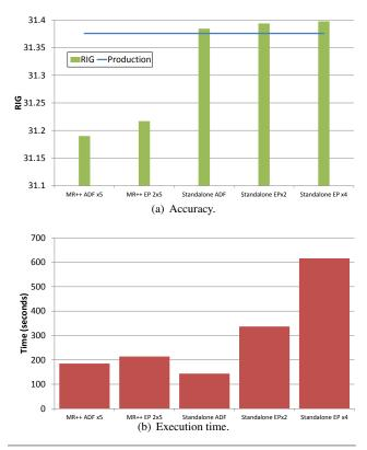
**Figure 2.** Accuracy and execution time for AdPredictor on 40 million click dataset.
