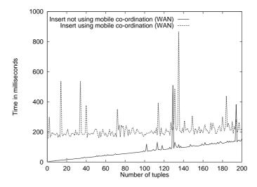
(a) Insert using mobility and not using mobility over a WAN.
