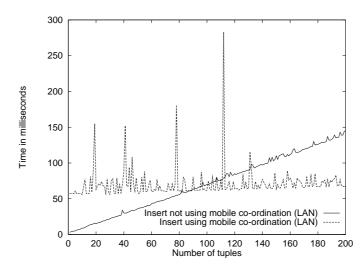
(a) Insert using mobility and not using mobility over a LAN.
